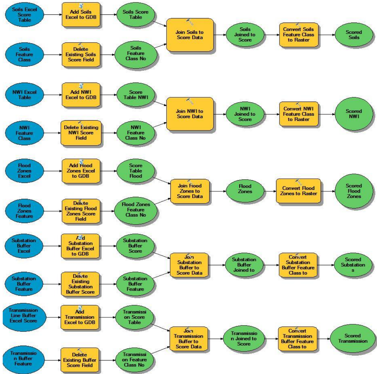
Figure 4 - The data processing model to prepare individual datasets to be used in the Cost-Weighted Overlay.
