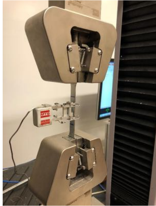
(b) details of extensometer and coupon
