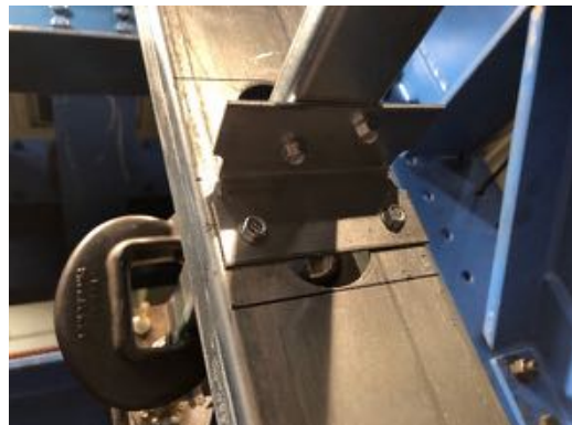
(c) detail of connection for bridging and stud
