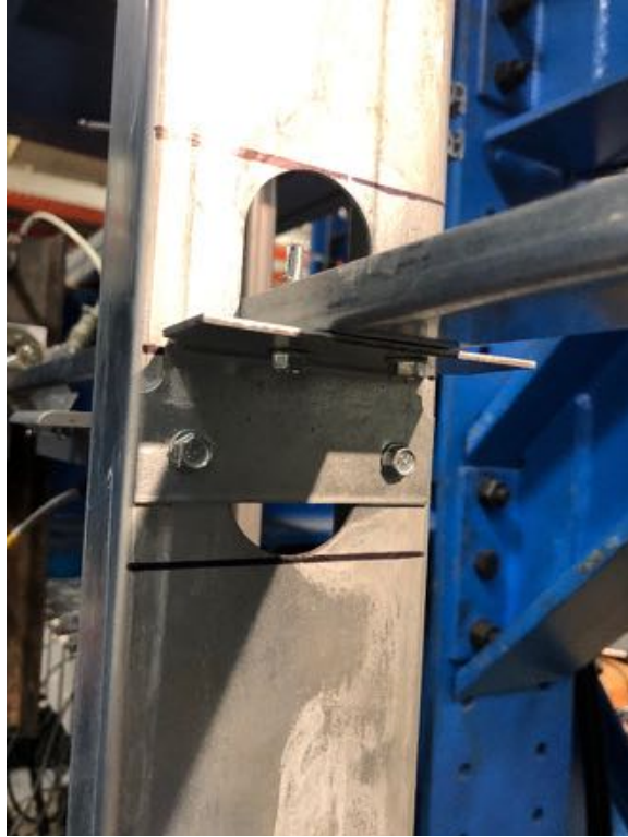
Figure 4. Connection of Clip to Stud with Bridging Channel
