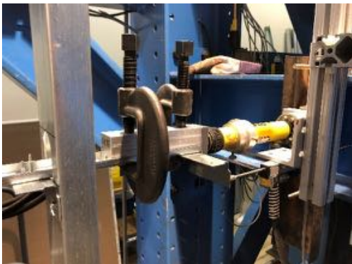
(b) detail of the end with jack and load cell
