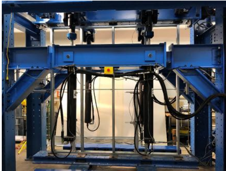
(a) all steel specimen, elevation view of AS-4 (blue is testing rig, silver is specimen)
