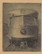
THE result of exhaustive wind-tunnel tests of conventional trolley car models revealed that at speeds of 70 and 80 miles per hour, 70 per cent of the total power was consumed in overcoming air resistance. Streamlining saves approximately 20 per cent of the power.
