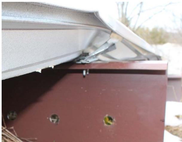
Figure A2-4 Clip damage of Specimen 2
