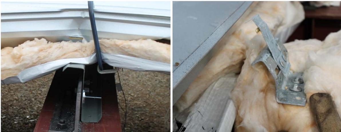
Figure A10-4 Clip damage of Specimen 10
