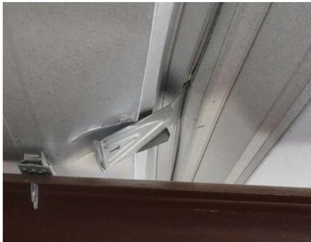
Figure A8-4 Clip damage of Specimen 8
