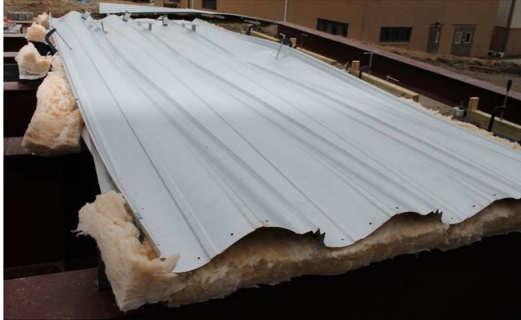
Figure A10-3 Deformed shape of Specimen 10
