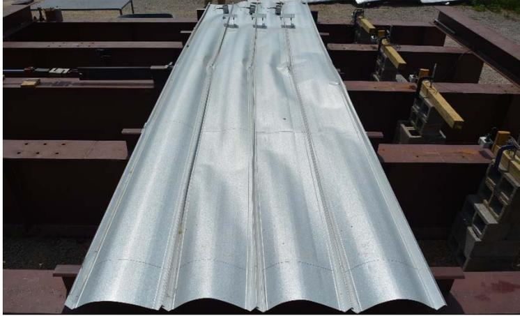
Figure A4-3 Deformed shape of Specimen 4
