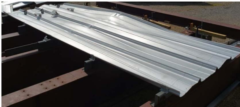
Figure A3-3 Deformed shape of Specimen 3
