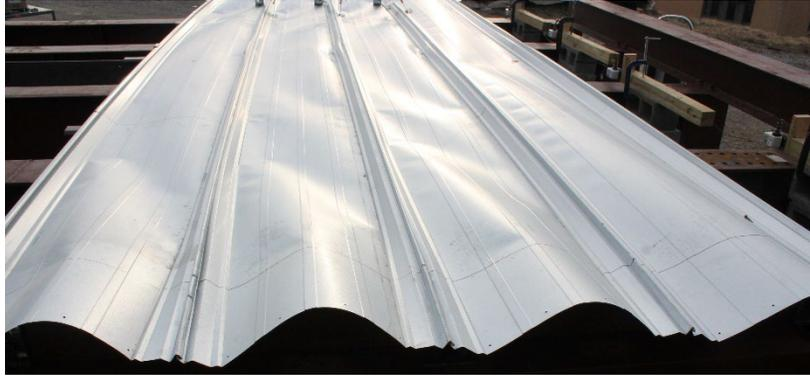
Figure 16 Typical deformed shape after panel buckling (from Specimen 7)
