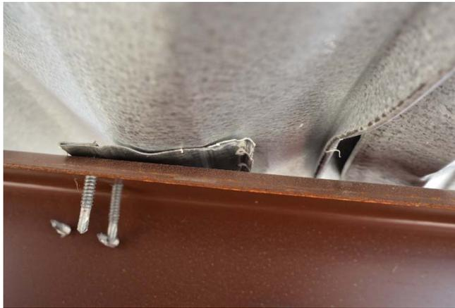
Figure A4-4 Clip damage of Specimen 4
