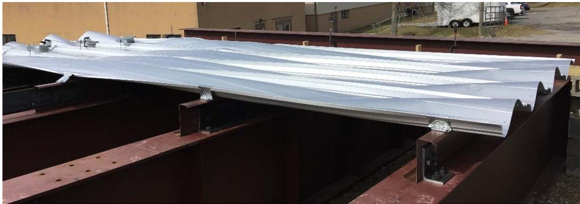
Figure A2-3 Deformed shape of Specimen 2
