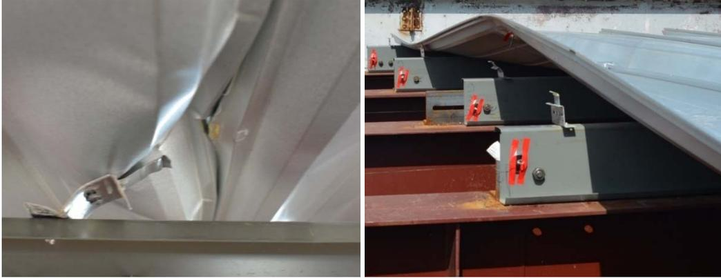
Figure A3-4 Clip damage of Specimen 3
