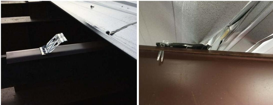
Figure A1-4 Clip damage of Specimen 1
