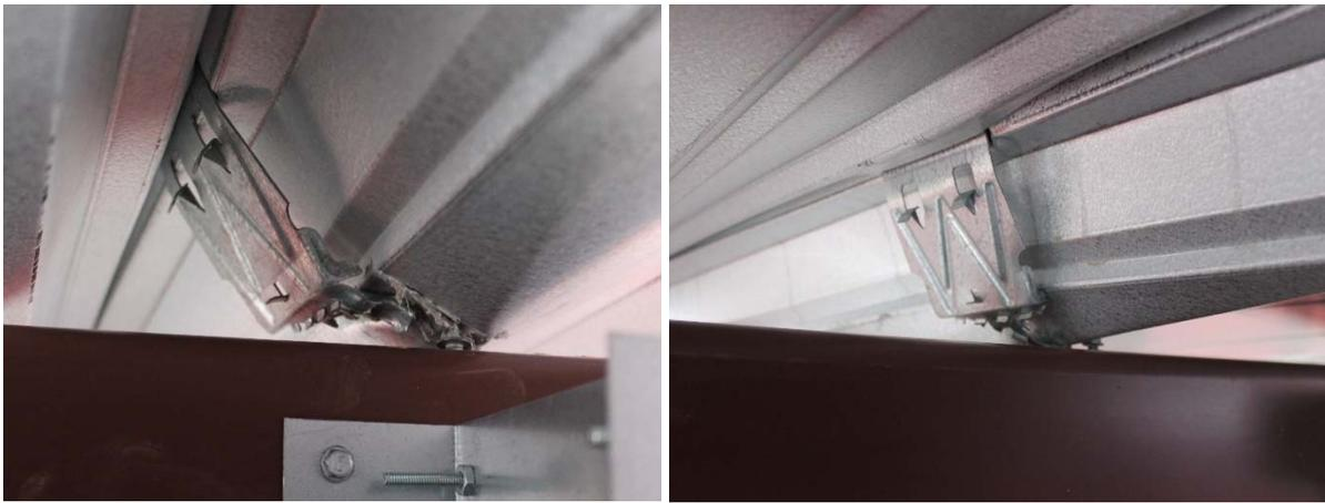
Figure A7-4 Clip damage of Specimen 7
