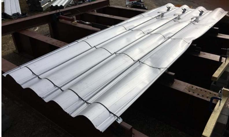
Figure A1-3 Deformed shape of Specimen 1
