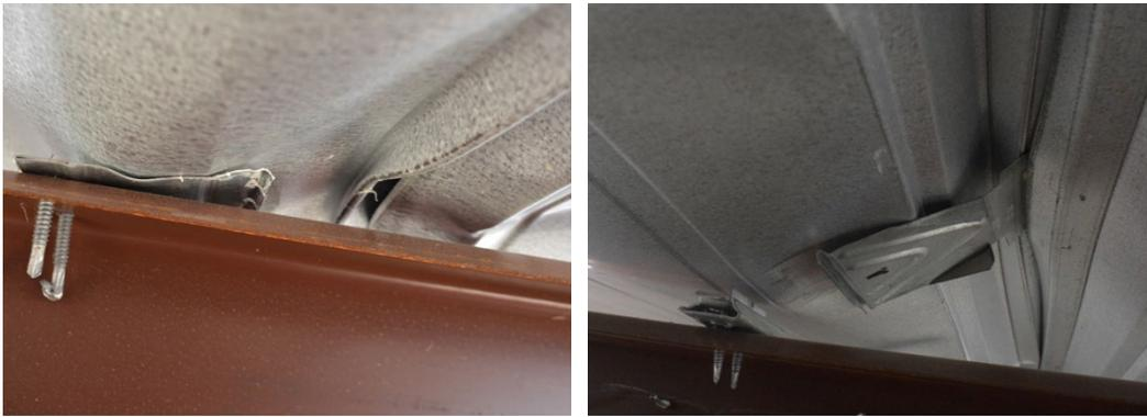
Figure 17 Mechanical detachment of clips from top (left) and bottom (right) (from Specimen 8)
