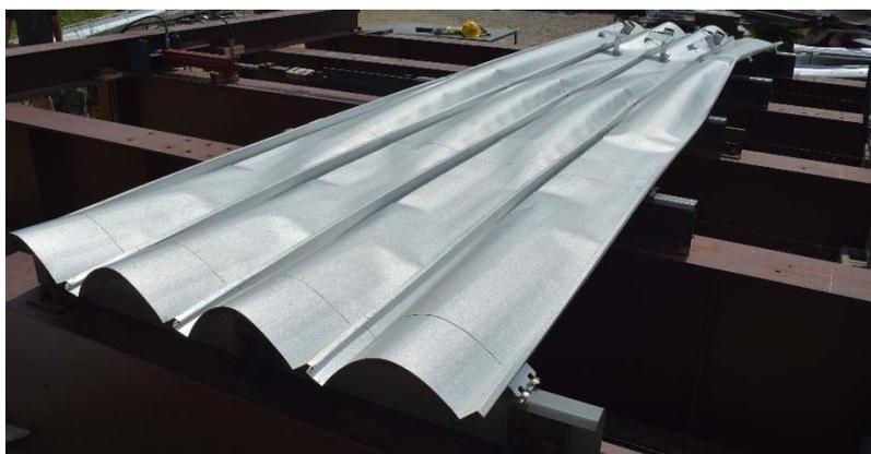
Figure A6-3 Deformed shape of Specimen 6
