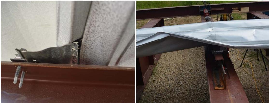
Figure A5-4 Clip damage of Specimen 5
