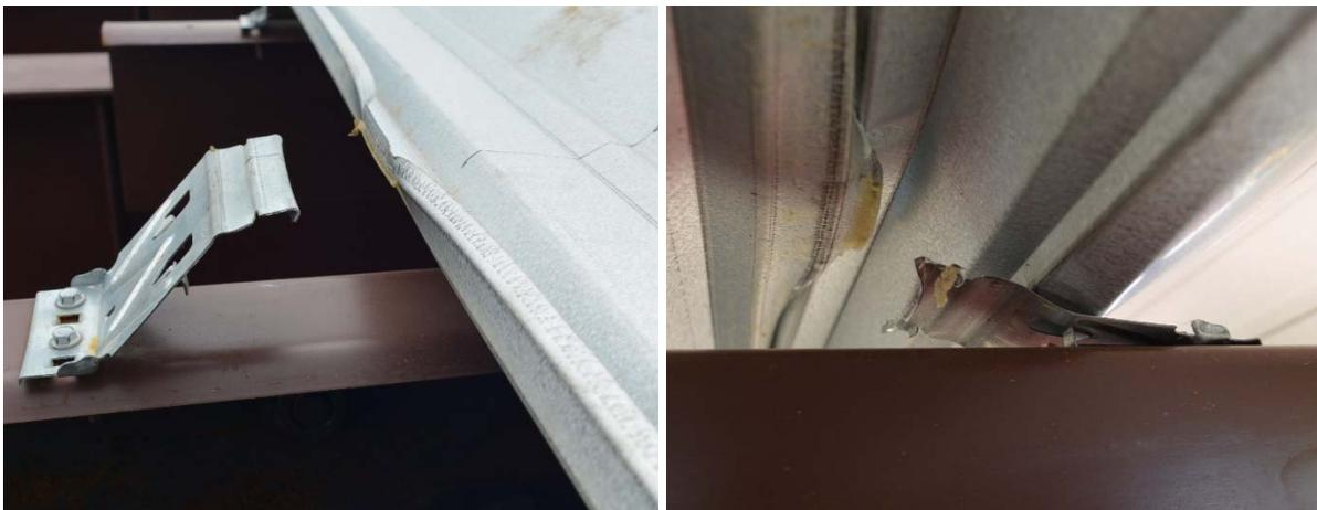
Figure A11-4 Clip damage of Specimen 11
