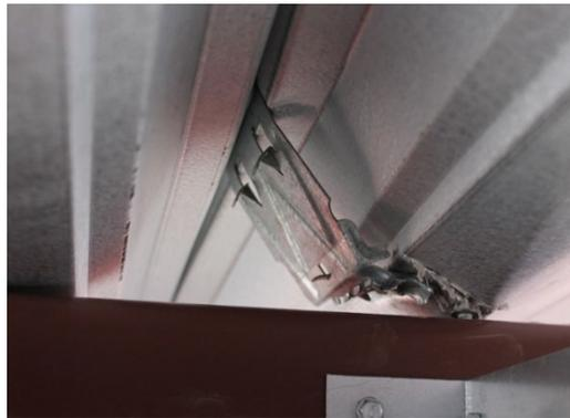
Figure 18 Tearing of clip material at the bottom (from Specimen 7)
