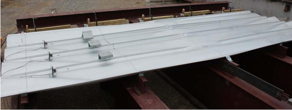
Figure A7-3 Deformed shape of Specimen 7
