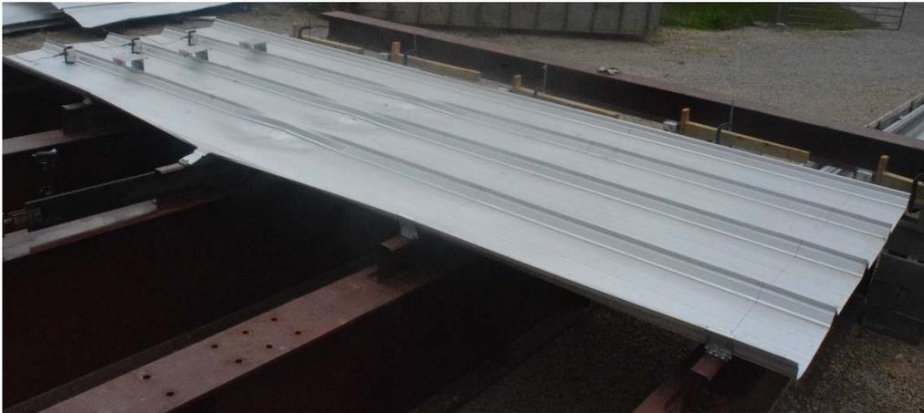
Figure A8-3 Deformed shape of Specimen 8
