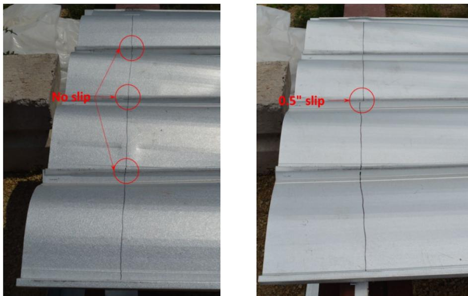
Figure 34 Slip between adjacent panels (left: Specimen 4; right: Specimen 5)
