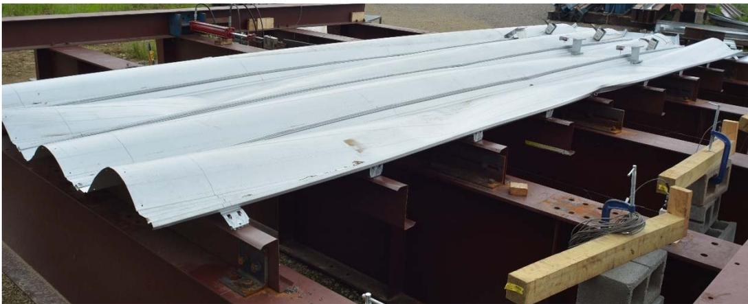
Figure A11-3 Deformed shape of Specimen 11
