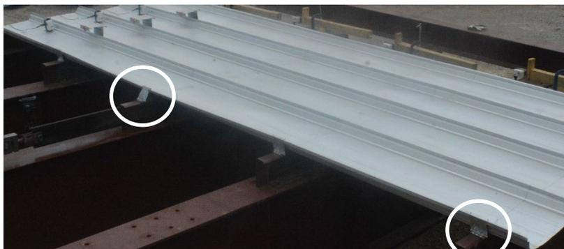
Figure 15 Typical deformed configuration with clip bending (from Specimen 7)
