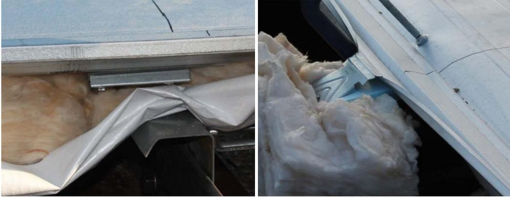
Figure A9-4 Clip damage of Specimen 9
