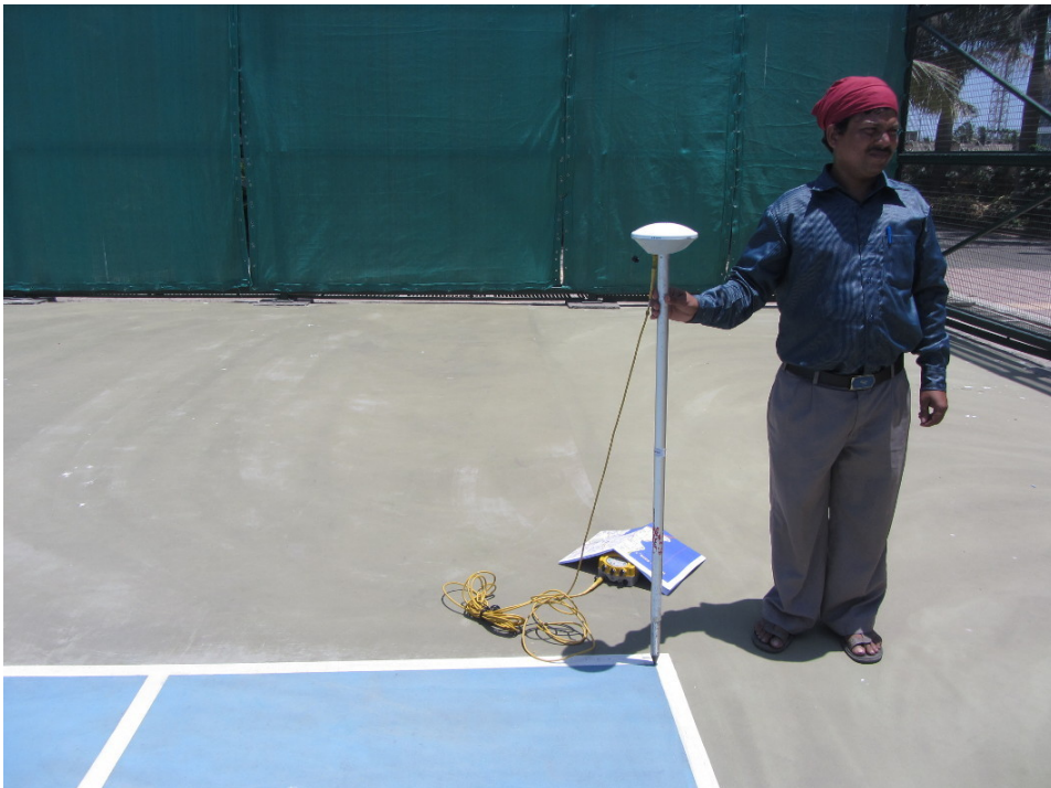
Figure 4: A survey team member holds the GPS device to record the co-ordinates of a point on the corner of a tennis court. In order to get the co-ordinates, the instrument has to be held perfectly still for several minutes. At his feet, one can see a reference map indicating all the roads in the area.
