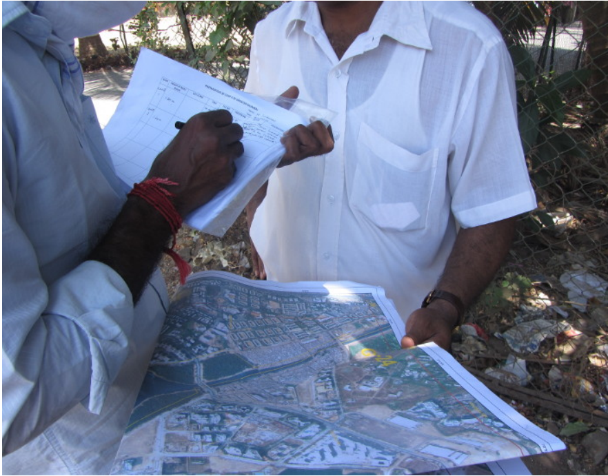
Figure 7: Surveyors make a record of all points on reference maps and on a log sheet.
