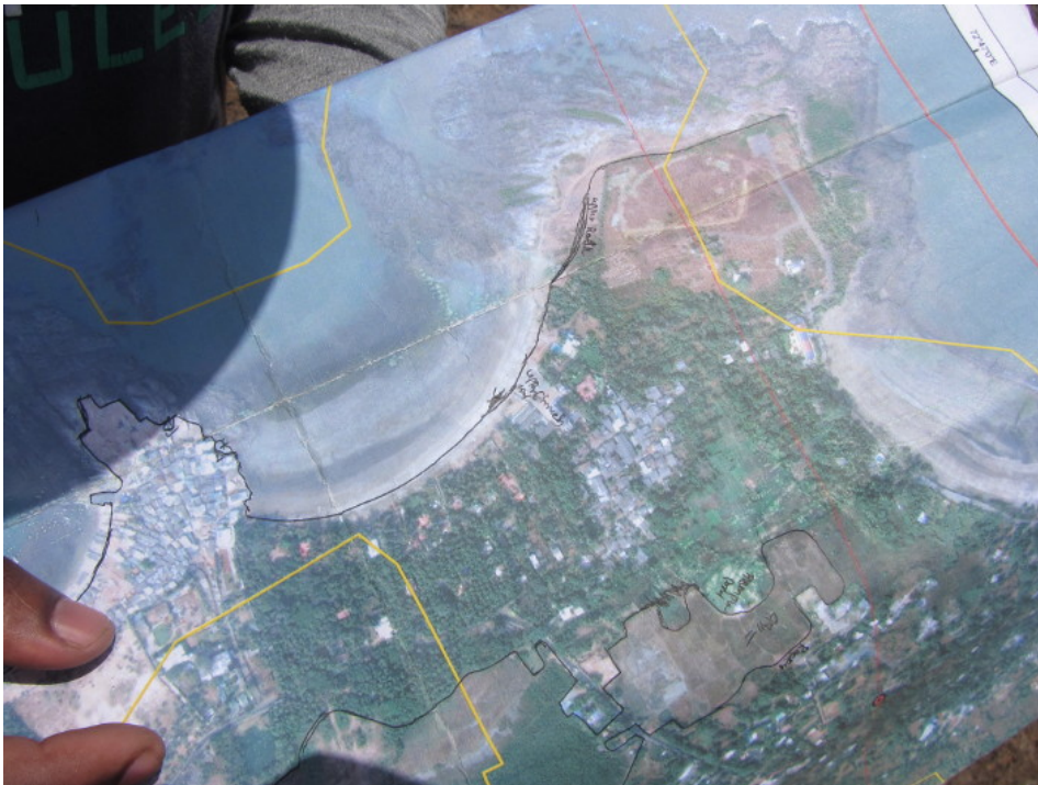
Figure 12: While mapping the HTL, the surveyors maintain a sketch of the features along the coast on the reference map.
