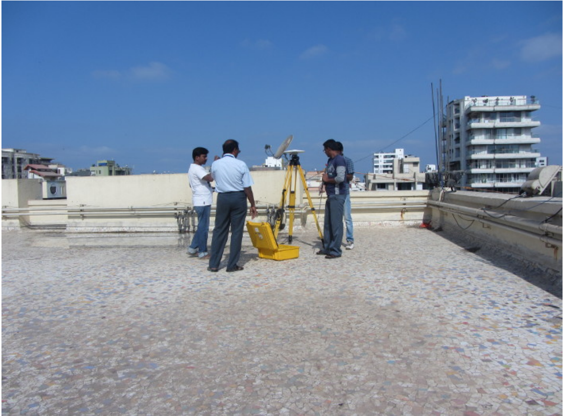
Figure 14: This picture shows the team of surveyors from Anna University in the process of establishing a main station on a terrace.
