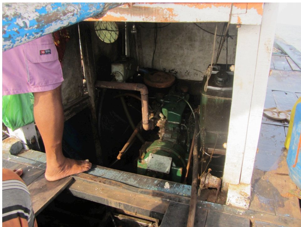
Figure 82: The picture above shows a retrofitted diesel engine typically used on boats. The engine is attached to the tiller that allows the pilot to steer the boat.
